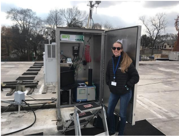
Metro Nashville Air Technician Morgan Dickie doing regular checks on her rooftop TEOM site with her Model 8872. The site was later changed to a T640 using Direct Poll, so the logger was eliminated from the site.
